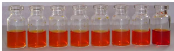
Fig. 5 (color online). Color changes are seen by naked eye for the complex Ru-L 1 ( 10^{-3} mol L -1 ) in 0.1 mol L -1 TBAP/CH 3 CN solution upon increasing [Na + ] from 0 to 0.1 mol L -1 (from right to left).
